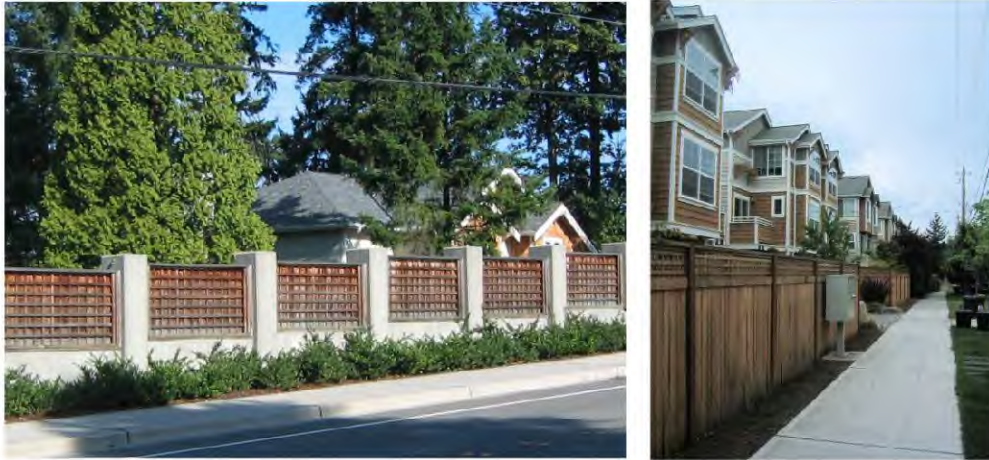
Figure 5.C.9-2. Fences that prevent visibility from public ROW and open spaces can decrease security.
