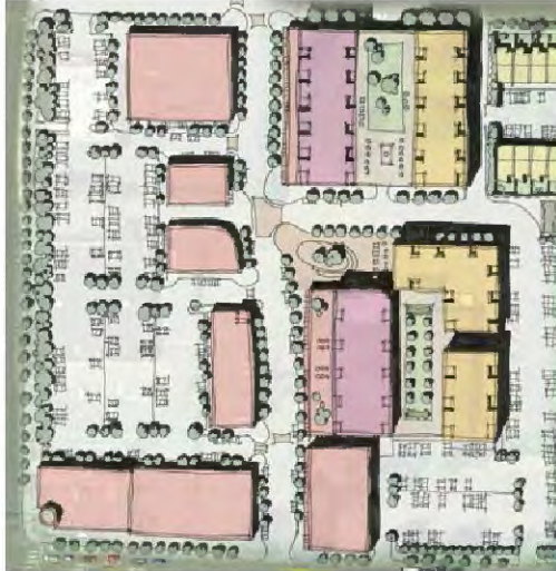
Figure 3.B.4.2-1. Pedestrian-oriented access streets are usually needed to provide good circulation to and through large sites.
