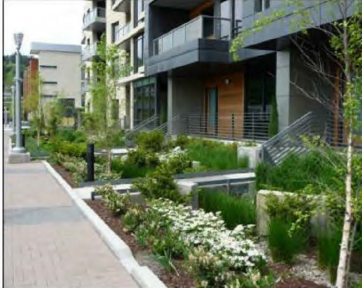
Figure 2.B.7.1-1 A preferred method of handling stormwater is through retention systems, such as rain gardens, incorporated as site amenities. Other low-impact development techniques are encouraged, and in many cases, required.
