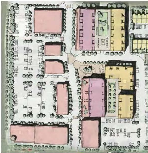
Figure 2.B.4.2-2 pedestrian-oriented access streets are usually needed to provide good circulation to and through large sites.
