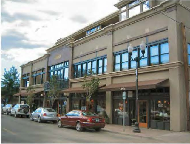
Figure 2.E.3.1-2. Example of a well articulated building. Note how the awnings, window divisions, pilasters columns and cornice line all serve to divide up the façade into smaller segments without disrupting the unity of the overall design.
