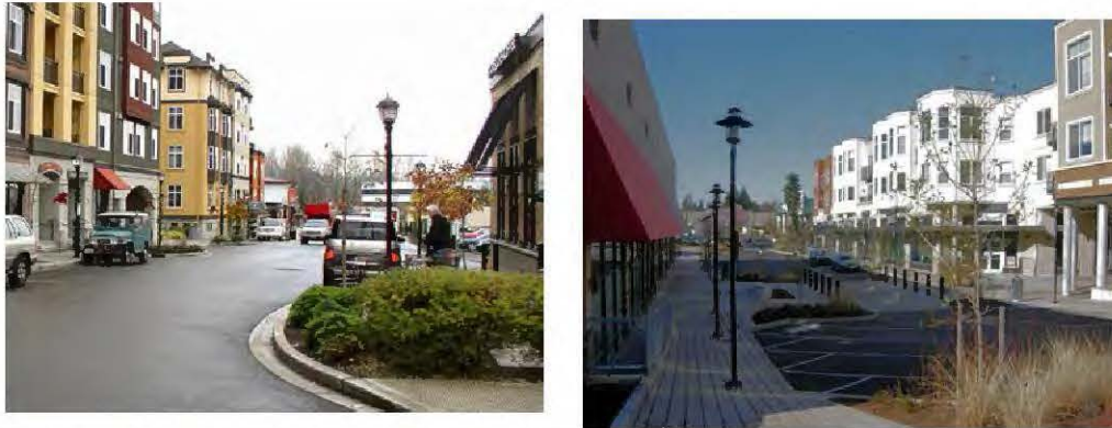
Figure 2.B.4.2-1. Two internal road examples. Juanita Village's internal roadways (left) are one model for circulation on large sites. Note the on-street parking, crosswalks, wide sidewalks, street trees, signage, and pedestrian lighting. The example on the right features a narrower road section with pedestrian amenities and crossing.
