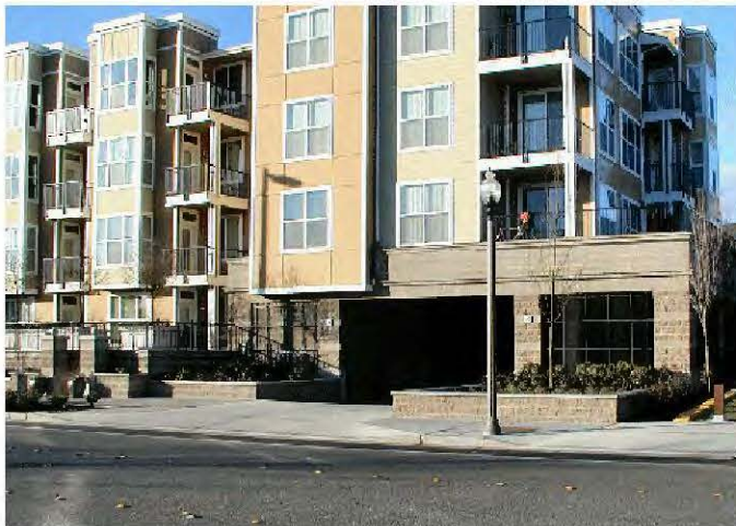
Figure 2.E.10.1-3. Design parking garages to obscure the view of parked cars. Note the landscaping that separates the garage from pedestrians.
