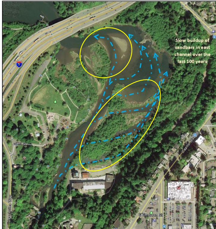
Figure 10. Showing sand bar islands in the area north of the Old Brewhouse site created by flow channel eddies (in blue dashed lines) formed by the I-5 Bridge constriction.
