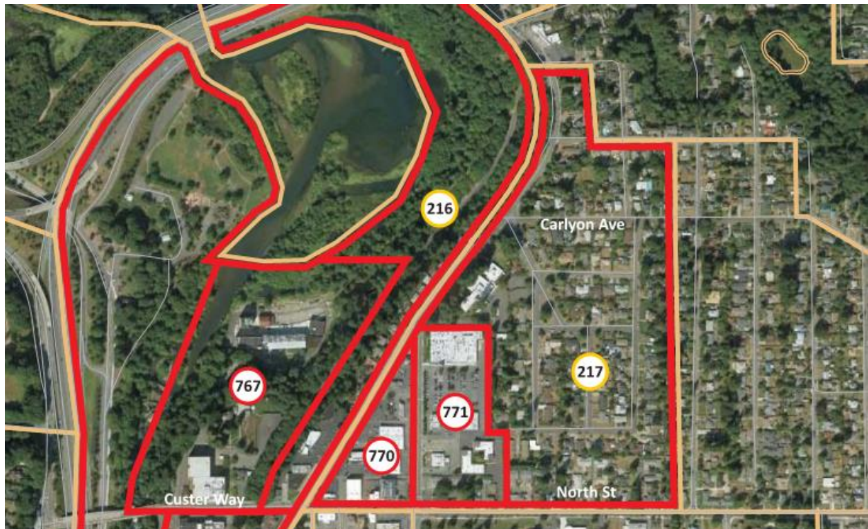
Figure 4. Traffic Analysis Zones (TAZs) Used in Travel Demand Modeling for the Brewery District Plan
