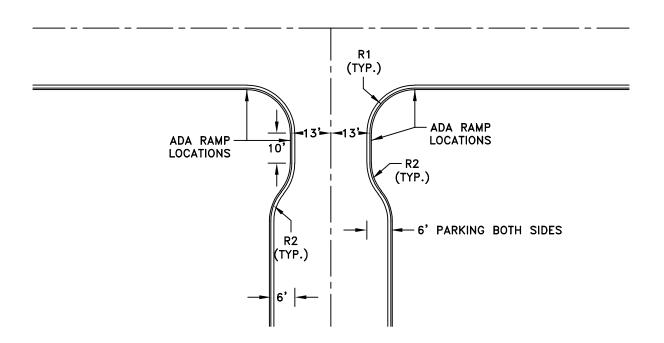
RETURN RADIUS R=15 R=20 R=25 PLACE RAMP AT SHORTEST DISTANCE BETWEEN CURBS, PERPENDICULAR TO CENTER LINE OF STREET
