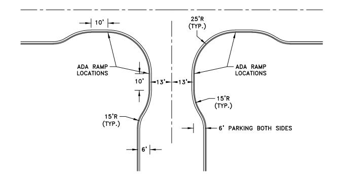
PLACE RAMP AT SHORTEST DISTANCE BETWEEN CURBS, PERPENDICULAR TO CENTER LINE OF STREET
