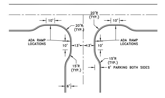
PLACE RAMP AT SHORTEST DISTANCE BETWEEN CURBS, PERPENDICULAR TO CENTER LINE OF STREET
