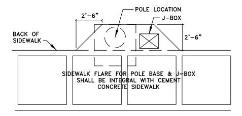
CITY OF TUMWATER, WASHINGTON DEPT. OF PUBLIC WORKS SHALLOW FOUNDATION **DETAIL** DWG. NO. APPROVED BY: **ST-15** CITY ENGINEER DWG. BY CK'D BY NOT TO DES. DATE **SCALE** PW PW MW JAN. 2015
