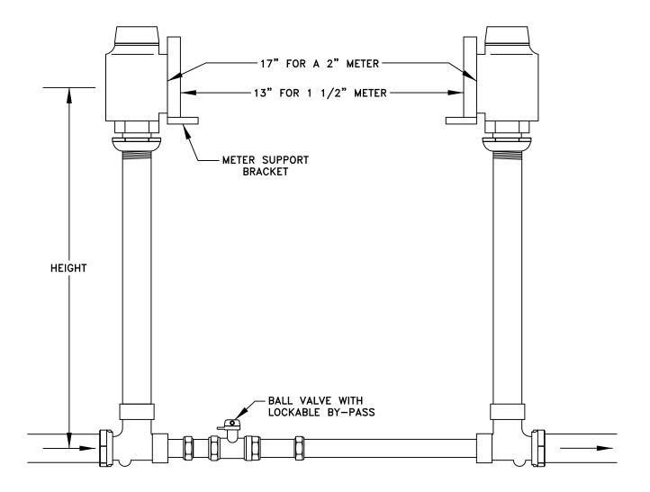
HEIGHT FOR 1 1/2" METER FOR 2" METER CATOLOG NUMBER: CATOLOG NUMBER:
