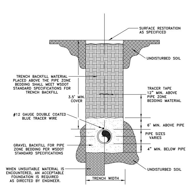
MAXIUM TRENCH WIDTH AT TOP OF PIPE: I.D. PLUS 30" FOR PIPE 15" AND UNDER. (1.5 XI.D.) PLUS 18" FOR PIPE 18" AND OVER.
