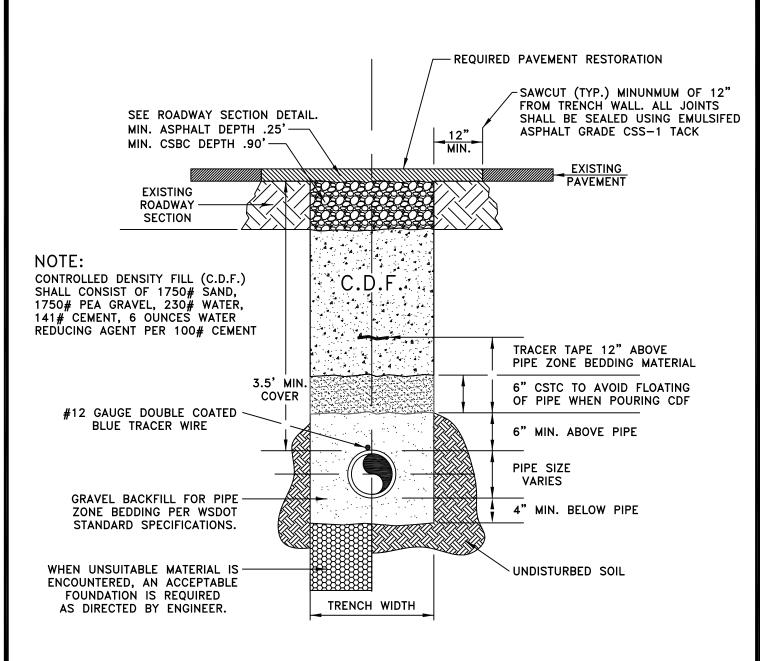
MAXIUM TRENCH WIDTH AT TOP OF PIPE: I.D. PLUS 30" FOR PIPE 15" AND UNDER. (1.5 XI.D.) PLUS 18" FOR PIPE 18" AND OVER.
