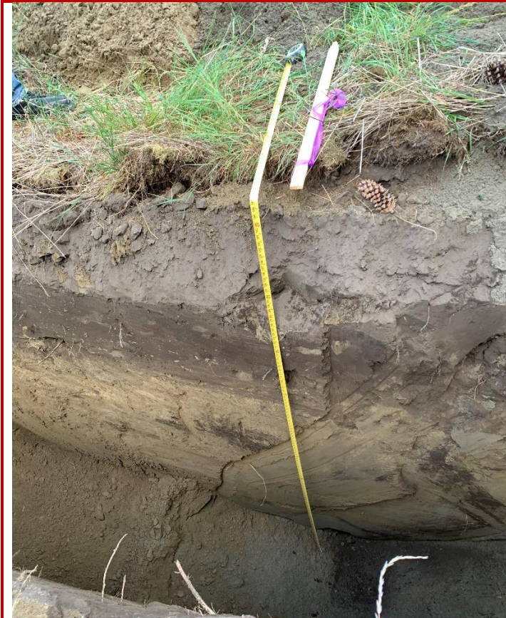
Photo 1: Sidewall of TP-04 showing 4-foot-thick surficial layer of fill over topsoil layer.
