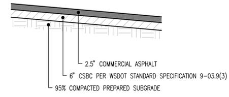
**TYPICAL ASPHALT PAVEMENT SECTION**
