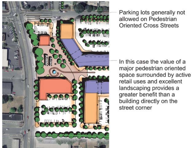
Figure B.1.1-2 Exception illustrating relaxation of the corner building requirement in B.1.1.f for an active public gathering space
