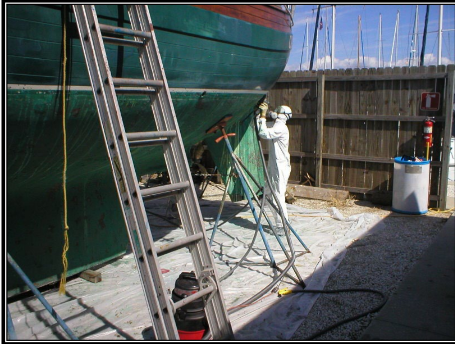
Figure 4.22. Drop Cloth Used During Hull Sanding.
