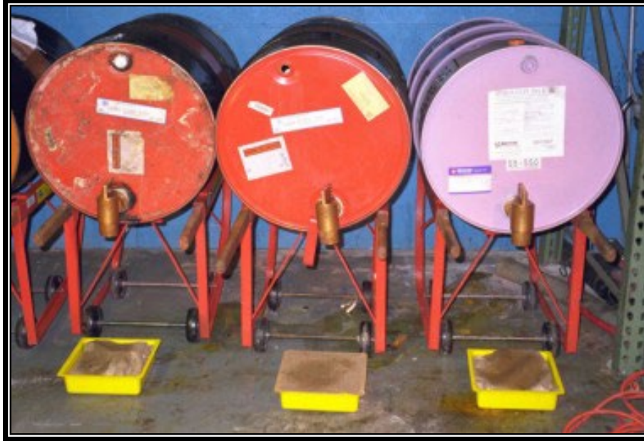
Figure 4.18. Mounted Containers with Drip Pans.
