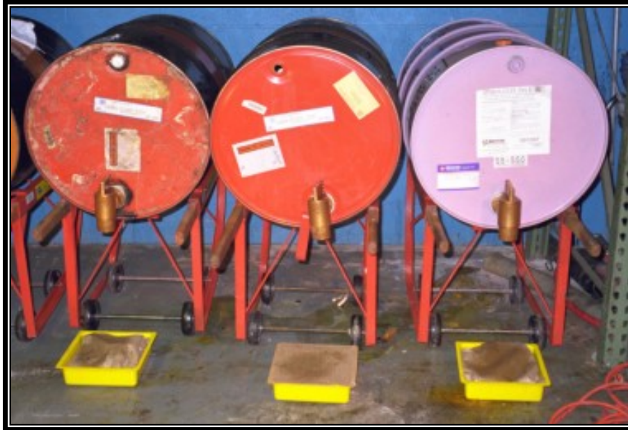
Figure 4.18. Mounted Containers with Drip Pans.
