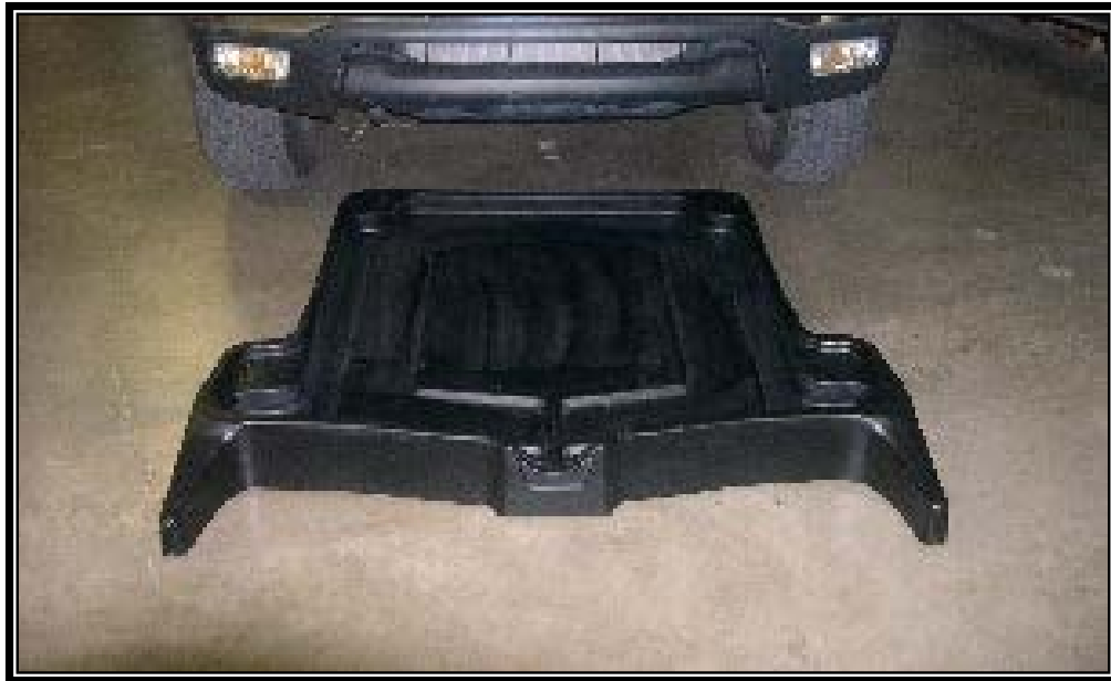
Figure 6.3. Drip Pan for Capturing Spills and Drips During Engine Repair and Maintenance.
